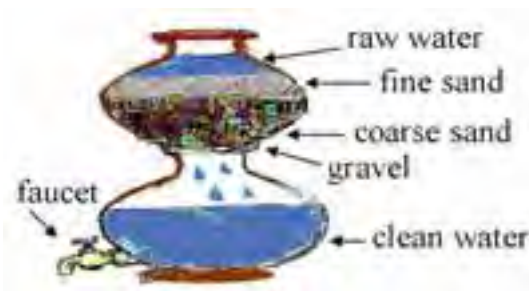
Figure 14.1 Household water filter using two clay pots placed on top of each other.
