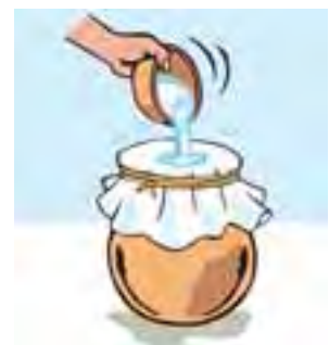
Figure 14.2 Cloth filtration. (Source: International Federation of Red Cross and Red Crescent Societies, 2008, Household water treatment and safe storage in emergencies )
