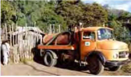
Figure 19.4 A tanker pumping out sludge from a septic tank or latrine. (Photo: Nicholas Watson)
