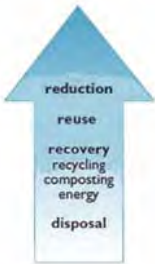
Figure 2.6 The waste hierarchy. Waste management options are listed in order of desirability from most desirable at the top to least desirable at the bottom.
