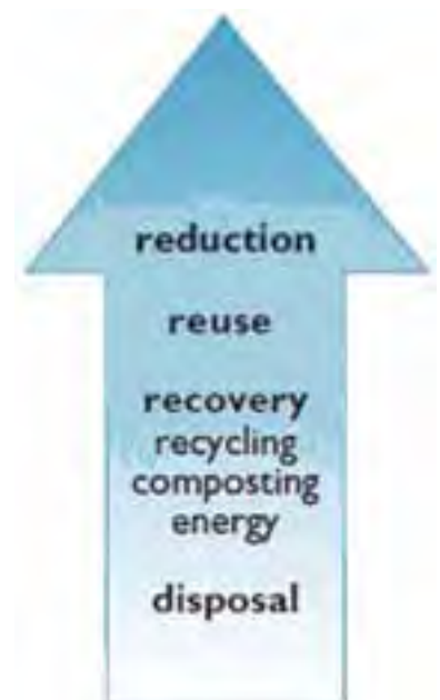
Figure 22.3 The waste management hierarchy. Waste management options are listed in order of desirability from most desirable at the top to least desirable at the bottom.
