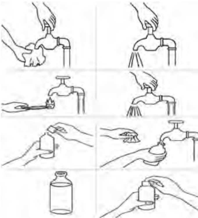
Figure 17.4 Procedures for sampling water from a tap. (Source: WHO, 1997, Guidelines for drinking water quality , Volume 3)
