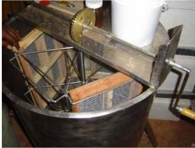
Photograph 32 - a centrifuge which can handle honey from the KTBH (placed in baskets) as well as the Langstroth hive
