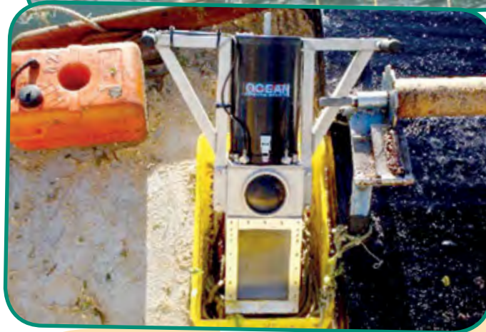
MANUAL DEPLOYMENT OF PROFILE IMAGER DURING A BIOLOGICAL SURVEY IN THE VENICE LAGOON IN ITALY.
