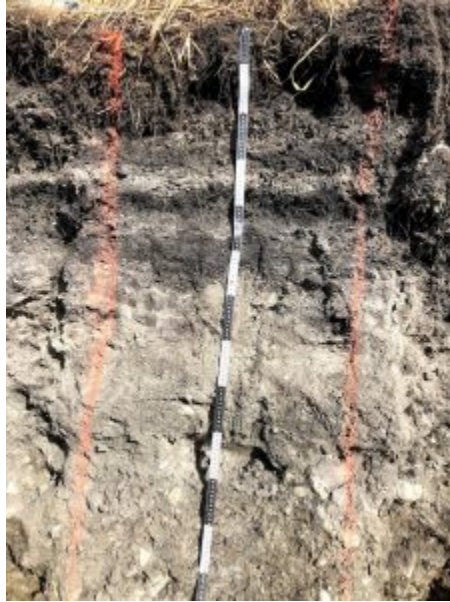
The alternating horizon color shows that water was a transporting force in this soil. Photo Credits Amber Anderson. Click to enlarge
