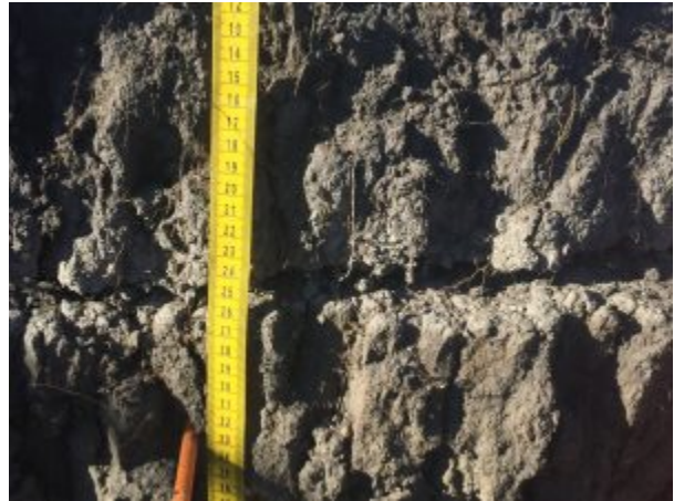
Columnar structure on a sodium-impacted soil in South Dakota. Significant sodium accumulation above the orange nail, around 25 cm of depth. Photo Credit: Amber Anderson. Click to enlarge
