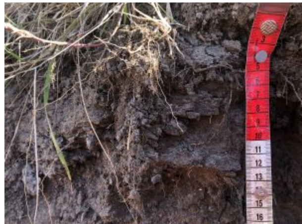
Although fragile, platy structure can be seen here, especially around 7-8 cm as the lines in the soil run horizontally rather than vertically. Photo Credit: Amber Anderson. Click to enlarge
