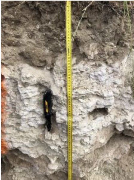
This aridisol in Southern California has significant calcium carbonate accumulation, cementing soil particles together. Unconsolidated soil can be seen under this cemented layer. Photo credit: Amber Anderson. Click to enlarge
