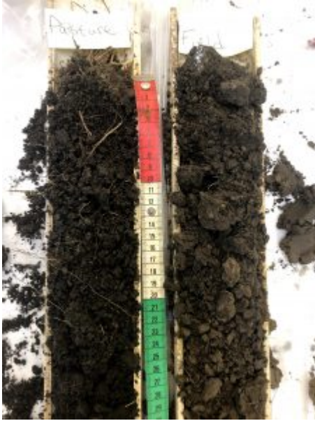
The impact of tillage can be seen here, with more blocky structure found in the right, cultivated core, while more granular structure is found on the left core, taken from a permanent pasture area. Photo credit Amber Anderson. Click to enlarge
