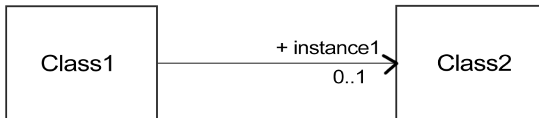
Figure 4.7 Unidirectional Association with Property Name and Target Multiplicity
