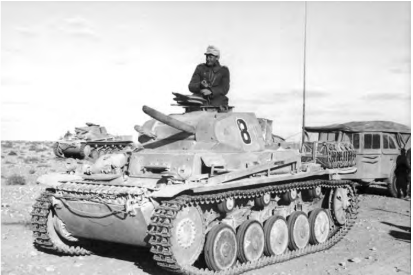
Panzer II of the 15th Panzer Division in North Africa used as Artillery Observation Tank.
