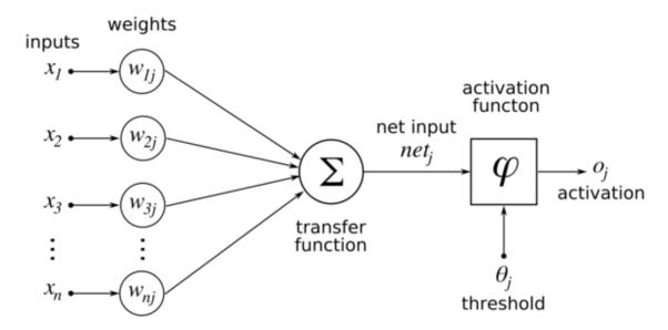
Figure 4.11 - Illustration of Artificial Neuron Processing
