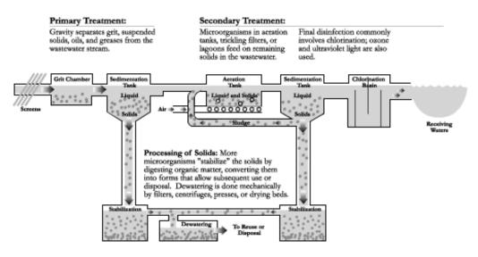
Figure 13.5 - Typical Processes in a Waste Water Treatment Plant
