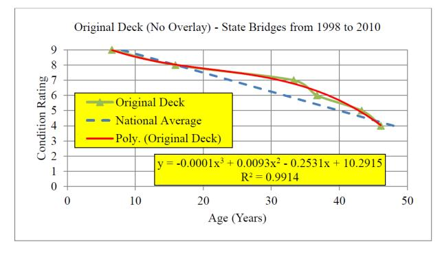
Figure 4.4 - Deterioration History and Model of Original Bridge Decks in Nebraska
