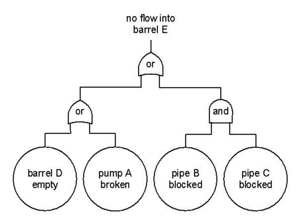
Suppose further that the estimated failure probabilities of the four sub-events are independent and are as follows (left to right in figure):
