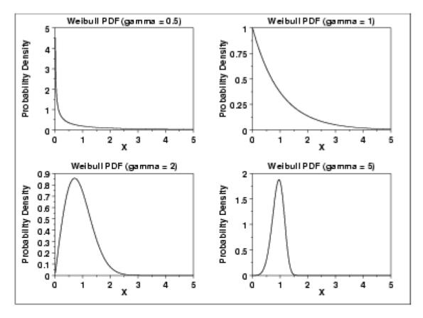
Figure 4.19 - Failure Probability Density Functions for the Weibull Distribution
