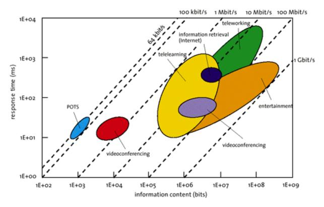
Figure 14.4 - New Applications Generate More Demand for Telecommunications
