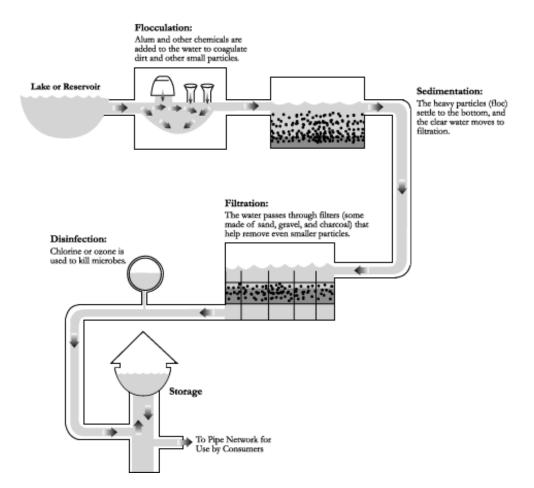
Figure 13.4 - Typical Processes in a Drinking Water Plant
