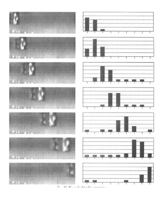
Figure 4.13 - Illustration of Output Activation for a Video Vehicle Identification System
