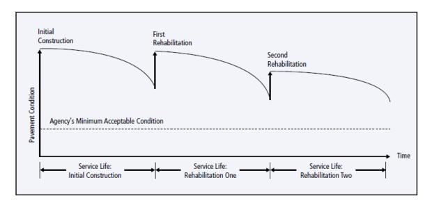
Figure 6.9 - Illustration of Life Cycle Costs for Pavement Construction and Rehabilitation
