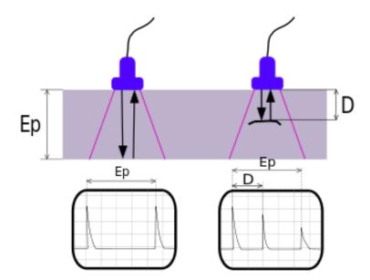
Figure 3.9 - Ultrasonic Structure Inspection
