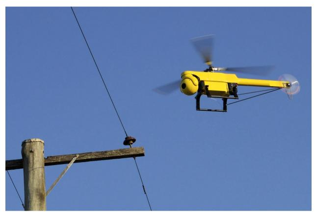
Figure 3.7 - An Unmanned Aerial Vehicle or 'Drone' used for Visual Inspection of Power Lines
