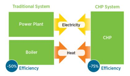
Figure 16.9 - Efficiency of Combined Heat and Power Systems
