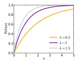
Figure 4.17 - Cumulative Failure Probabilities for Exponential Failure Models
