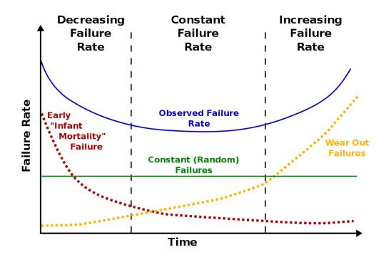
Figure 4.14 - Illustration of a Bathtub Curve
