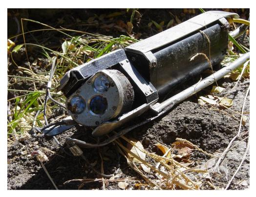
Figure 3.6 - A Video 'Pig' for Pipe Inspection
