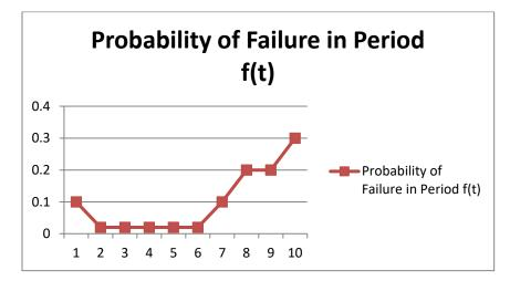
Figure 4.15 - Probability of Component Failure in Year t from Table 4.1 Data
