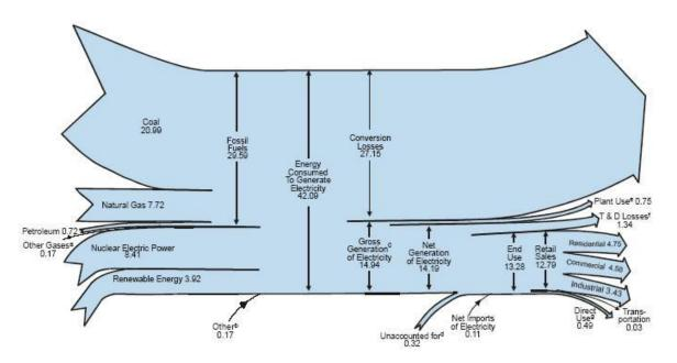
Figure 15.2 - US Electricity Flows, 2007, Quadrillion BTU
