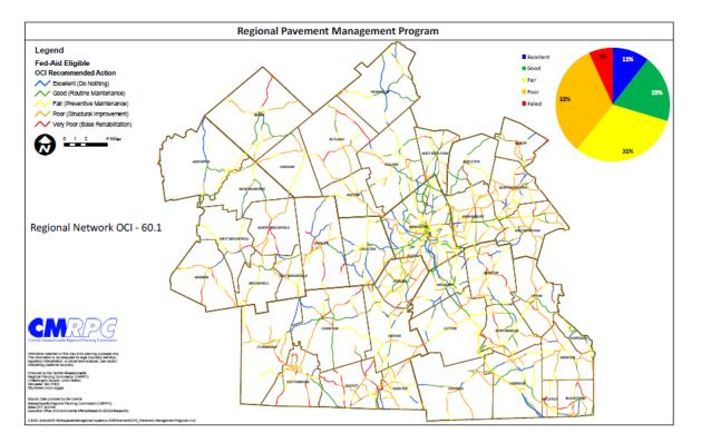
Figure 3.5 - Example Display of Pavement Conditions
