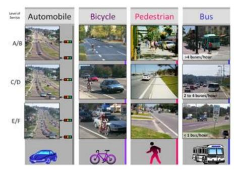
Figure 2.6 - Pictorial Examples of Level of Service A to F for Multiple Transportation Modes
