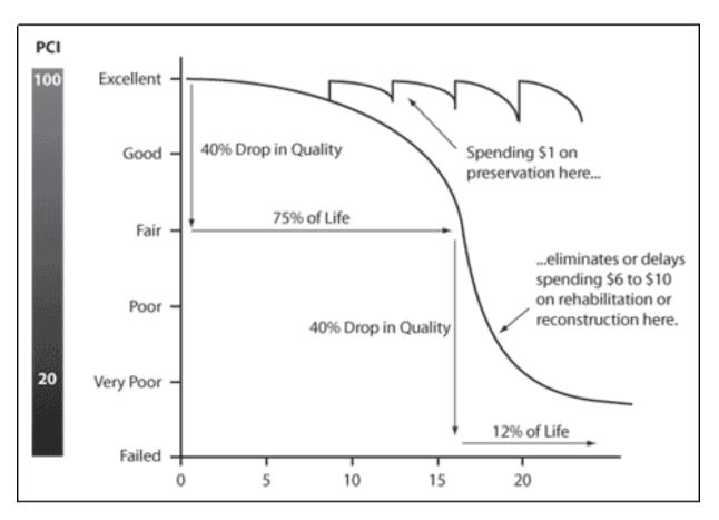
Figure 4.1 - Illustration of the Deterioration Hypothesis
