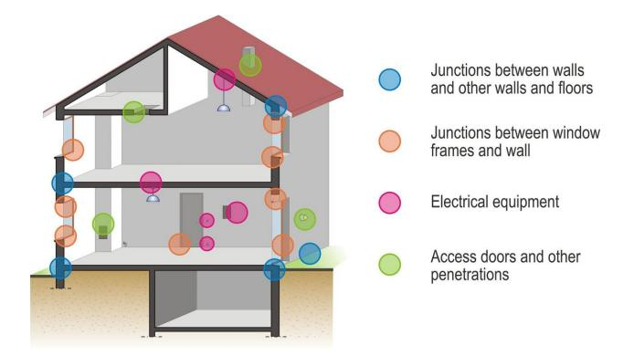
Figure 9.2 - Some Sources of Air Leaks in a Typical Building
