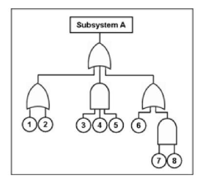
Figure 4.20 - Illustration of a Fault Tree with Eight Different Subcomponents or Events
