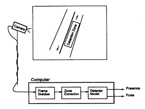
Figure 4.12 - Video Vehicle Identification System
