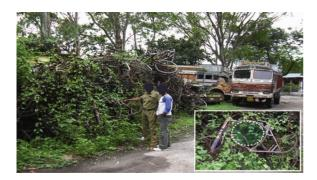
Figure 6.6: Bicycles and trucks confiscated from people caught illegally removing large logs from the forests. Note the circular modification in the cycle frame (Inset) made to hold large logs of teak wood.
