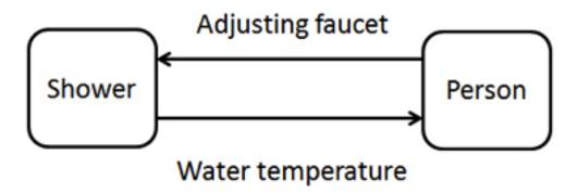
Figure 12.2: Hot water faucet adjustment from a systems perspective.
