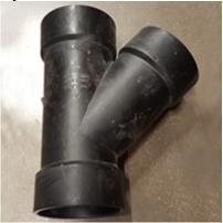
Wyes are Y-shaped fittings that allow one pipe to be joined to another at a 45 degree angle. Wyes are not used in water supply systems, but are common in DWV systems where hard turns slow the flow of waste.
