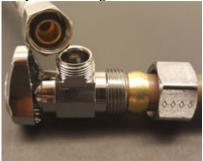
Compression fittings are sometimes used to install plumbing system components and make quick repairs on smooth outside diameter pipes like PVC and copper. Compression fittings require that a soft brass metal sleeve in copper applications, and Teflon or pliable washer in PVC applications, is compressed around the piping material by an adjustment nut to seal the fitting.
