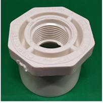
This fitting allows a pipe or fitting to be reduced to a smaller size and are made to be inserted into a pipe, inside slip, or female thread. Bushings outside diameter can be male thread or male slip with the inside diameter, being of the same style (slip or thread) as the outside, dictating the size the piping system is reduced to.
