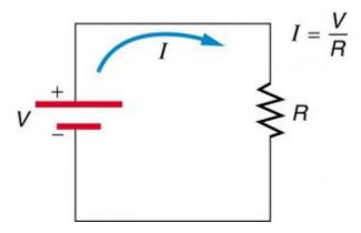
A simple electric circuit in which a closed path for current to flow is supplied by conductors (usually metal wires) connecting a load to the terminals of a battery, represented by the red parallel lines. The zigzag symbol represents the single resistor and includes any resistance in the connections to the voltage source. An interactive or media element has been excluded from this version of the text. You can view it online here: http://pressbooks.oer.hawaii.edu/ buildingmaint/?p=150
