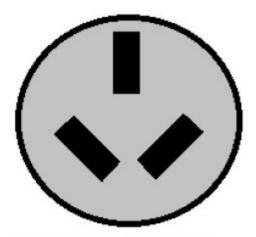
50 AMPERE, 3 POLE, 3 WIRE, 125/250 VOLT, NEMA 10-30R PERMITTED PRIOR TO 1996 NEC ®
