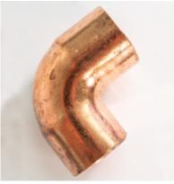
Elbows normally create a 90° or 45° change in direction of a piping system. 22-1/2° fittings are also available for some piping systems. Depending on the material, elbows come in female slip-to-female slip, female slip-to-female slip, slip-to-female thread, slip-to-male thread, PVC and Copper female slip-to-male slip elbows are referred to as street elbows and they are used for close turns and swivel to fit connections.
