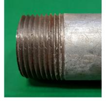
American standard thread used in pluming and piping systems. It may also be referred to as MPT or MNPT for male external threads and FPT or FNPT for female internal threads. A thread sealant of some type should always be used to obtain a leak free seal (except for NPTF).
