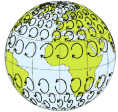
In the Northern Hemisphere the Coriolis force acts to the right (clockwise motion), while in the Southern Hemisphere the Coriolis force acts to the left (Counter-Clockwise).
