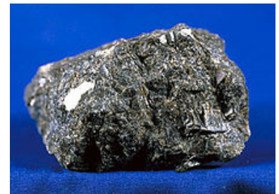
Gabbro is a dark mafic rock, with large crystals. Gabbro is common in oceanic crust beneath the ocean floor.
