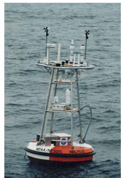
Ocean instrumentation buoy, typical of those used by the Tropical Atmosphere Ocean Project.
