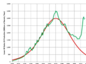
Oil production peaked in the early 1970s in the United States, the second increase during 2004-2010 was due to fracking and other technology.
