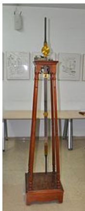
A pendulum used to measure gravity at different locations on the surface of the Earth.
