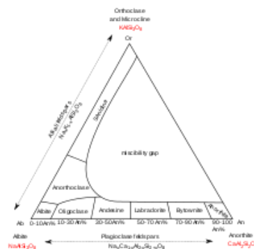
The feldspar group of minerals, showing end members (potassium, sodium, and calcium)
