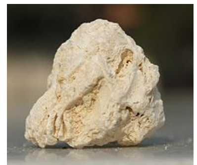
A piece of limestone composed of calcium carbonate from tiny fossil organisms.
