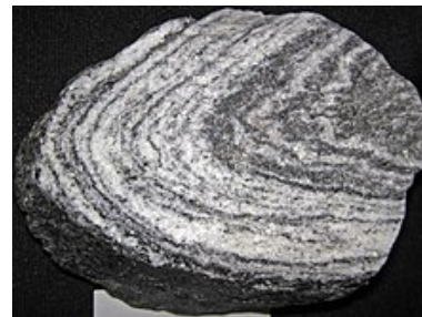
Example of foliation caused by intense pressure and temperatures that form metamorphic rocks.
