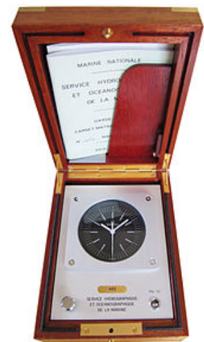
A Modern Marine Chronometer, which is a highly accurate clock used to tell longitude.
