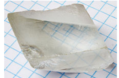
A crystal of calcite which produces a double image because the light bends as it passes through the crystals.
