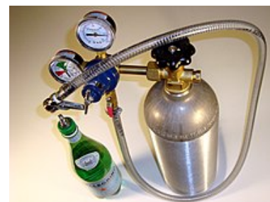
Carbon dioxide gas is added to water to carbonate it, resulting in sparkling or soda water found in many "soft" drinks. It significantly lowers the pH of the water in the process.
