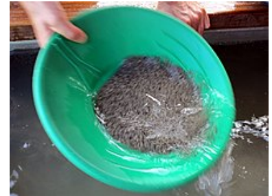
Panning for gold, because of its high specific density gold will sink, and remain within in an agitated pan.
