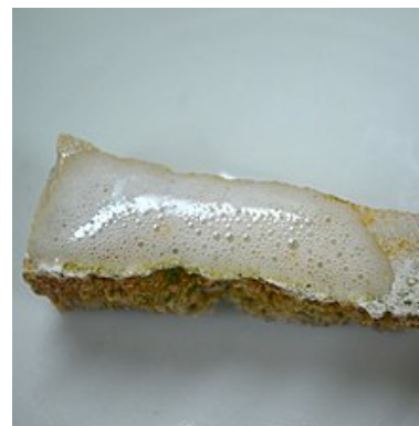
Reaction of hydrochloric acid to the mineral calcite.
