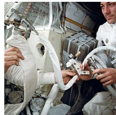
The "mailbox" rig improvised on the Apollo 13 command module's square carbon dioxide scrubber cartridges to fit the lunar module, which took a round cartridge. This allowed the carbon dioxide levels to return to normal.
