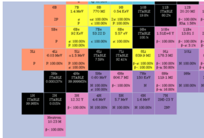
Close up of base of the Chart, showing isotopes from Hydrogen to Boron. Note that the axis is reversed than above the number of Protons is on the vertical axis (y-axis) and number of Neutrons on the horizontal axis (x-axis), such that all atoms with 1 proton are H, 2 are He, etc.
