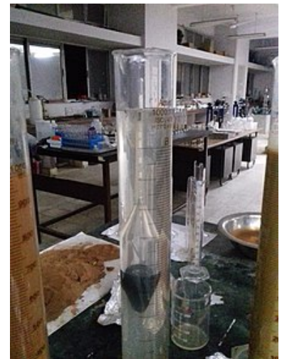
A hydrometer measures the density of the water (or other liquid) by floating a standard weight.
