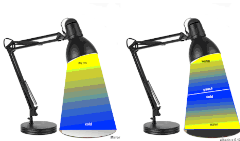
Example of heat absorption resulting in a gradient of temperatures below a lamp. If the surface is a perfect reflector, then the coldest zone would be above the surface, if the surface absorbs some of the heat the coldest zone would be somewhere between the lamp and the surface, this cold zone is called a pause.
