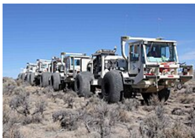
Thumper trucks produce waves in the subsurface that are recorded by geophones, to make a seismic profile of the materials under ground.
