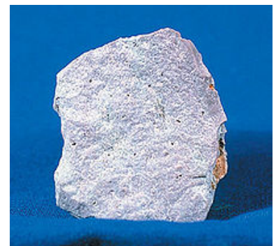
Rhyolite is a light colored rock that cooled quickly (extrusive), notice the small crystal sizes (aphanitic texture).
