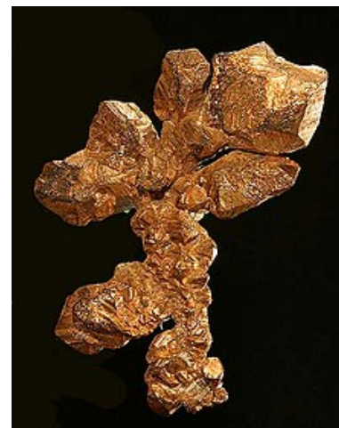
Native copper is an example of metallic bonding of Cu (copper) atoms, which is an excellent conductor of electricity, and ductile (bendable).
