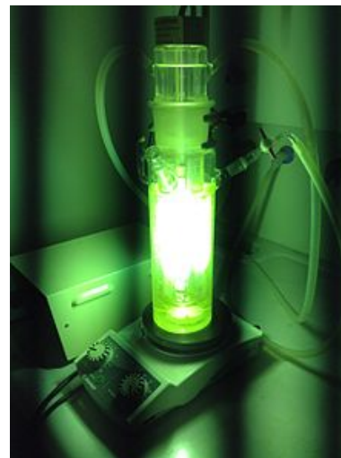
Photochemistry experiment using a mercury gas filled glass tube.
