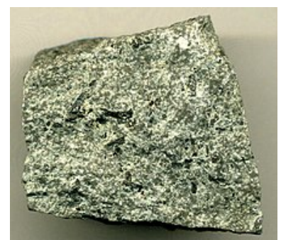
Andesite, which exhibits tiny crystals of both mafic and felsic minerals, and cooled quickly.
