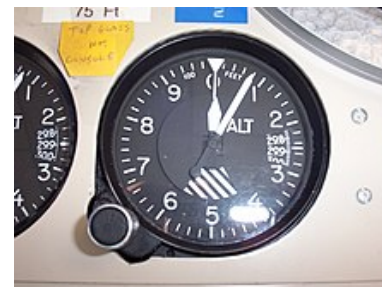
An altimeter on an airplane uses atmospheric pressure to determine how high in the air the plane is traveling at.
