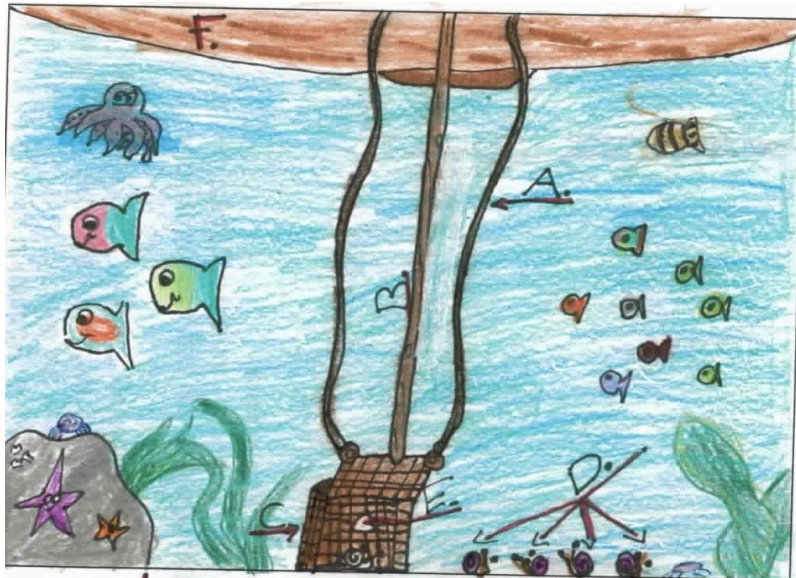
Figure 9.5 ▲ “The Super Catcher. A. 200 ft seal rope. B. 100 ft wood stick. C. 14 cm long/wide wood cage. D. Dentalia. E. Bait. F. Canoe bottom. Put bait in the cage. Close the door and grab the rope. Drop the cage till it hits the bottom. When you think there’s a dentalia, drop the stick that closes the door and pull the rope to get the cage.” Drawing by Grade 6/7 student (2007)
