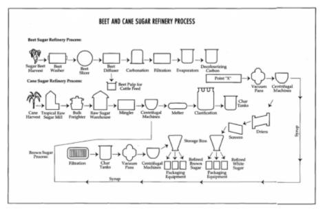
Figure 2. Sugar refining process.
