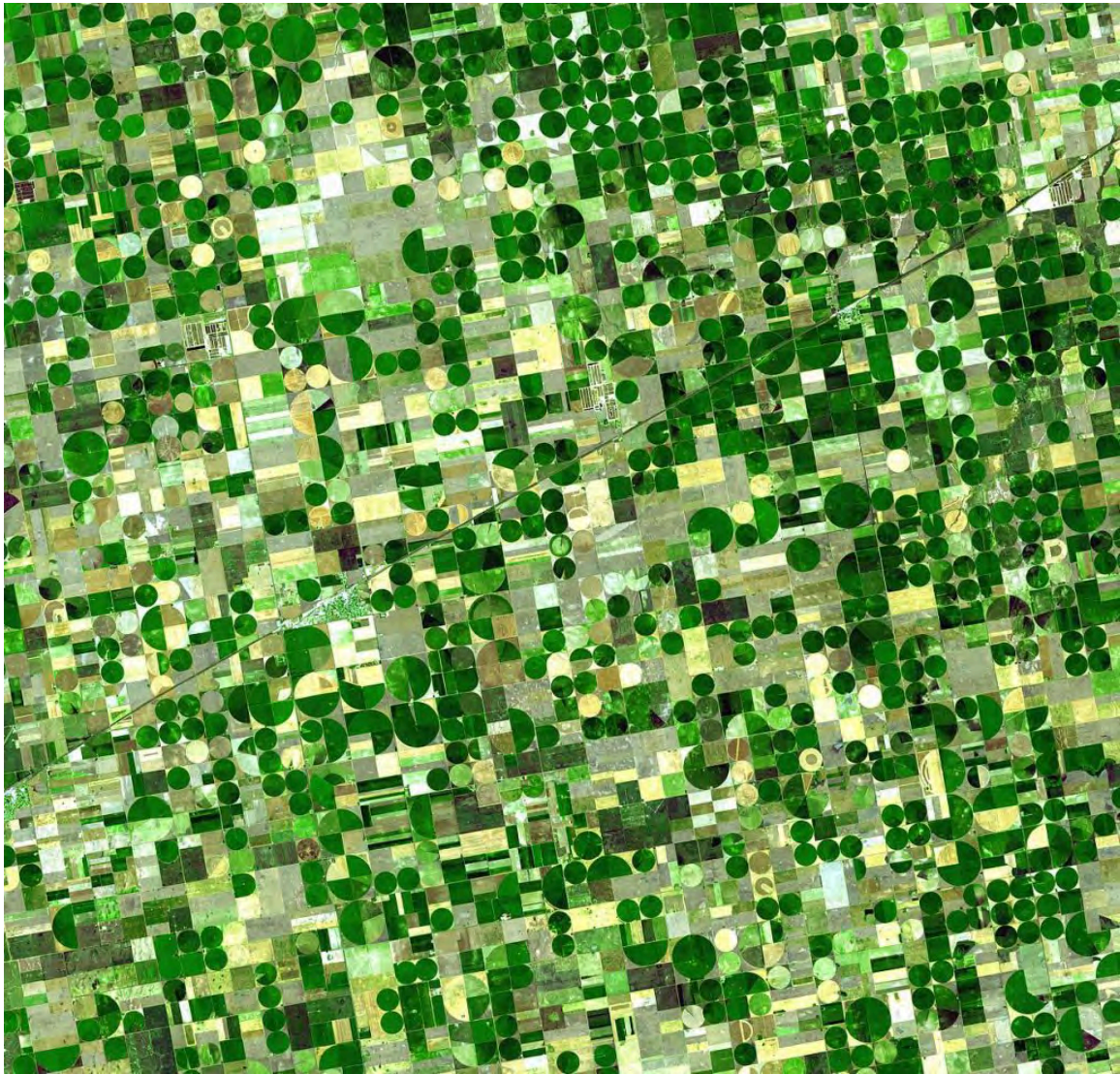
Fig. 6 Satellite view of Kansas cropland. The circles reflect the use of central pivot irrigation systems where a large boom circles around the water source. The boom is motorized to allow for its circular movement; water, supplied from a well, is pumped out of the boom and used to irrigate crops.
