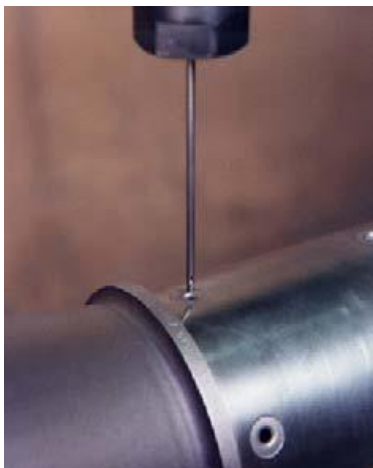
Figure 22 – Peening a turbine shaft oil hole (0.140" diameter)
