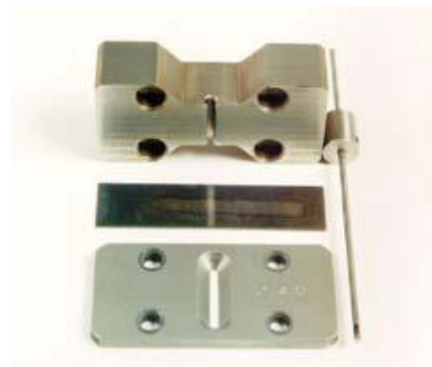
Figure 31 – Mask plate for 0.14" hole, simulated hole fixture, peened strip and small rotary lance.
