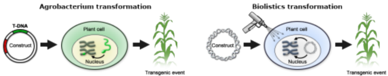
Fig. 12 Plant transformation by Agrobacterium or Biolistics methods. Each random insertion of the construct into the cell genome results in a transgenic event.
