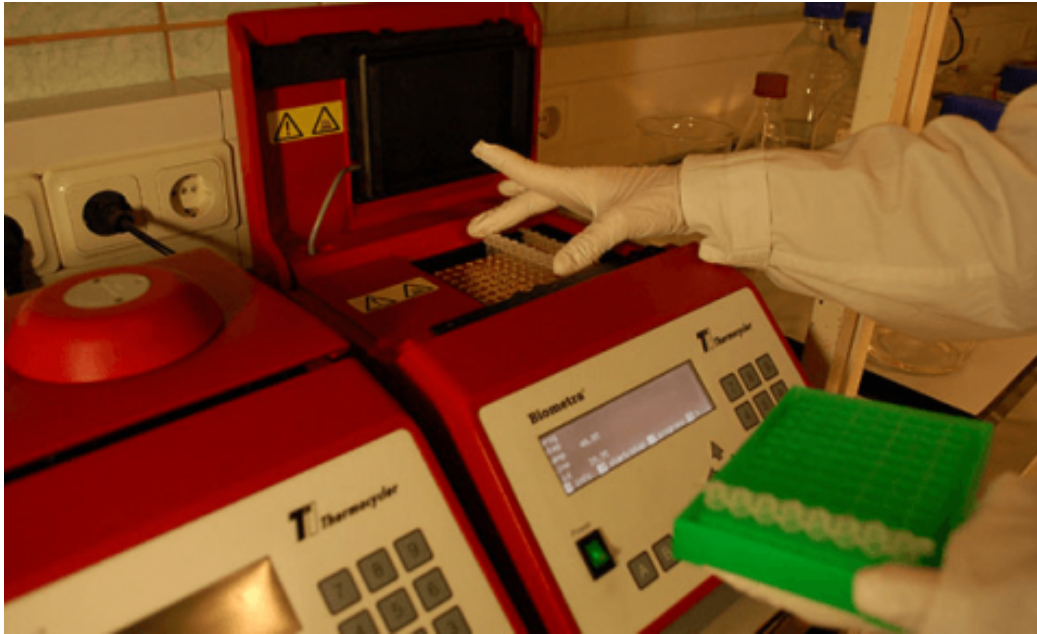
Fig. 17 A technician places a strip of eight PCR tubes into a thermal cycler at the University of Tartu in Estonia. Photo by Karl Mumm. Licensed under CC BY-SA 3.0 via Wikimedia Commons.
