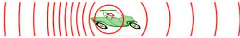
Figure 17.3: Doppler effect. The ripples made in the direction the car is moving are closer together than the ripples behind the car.
