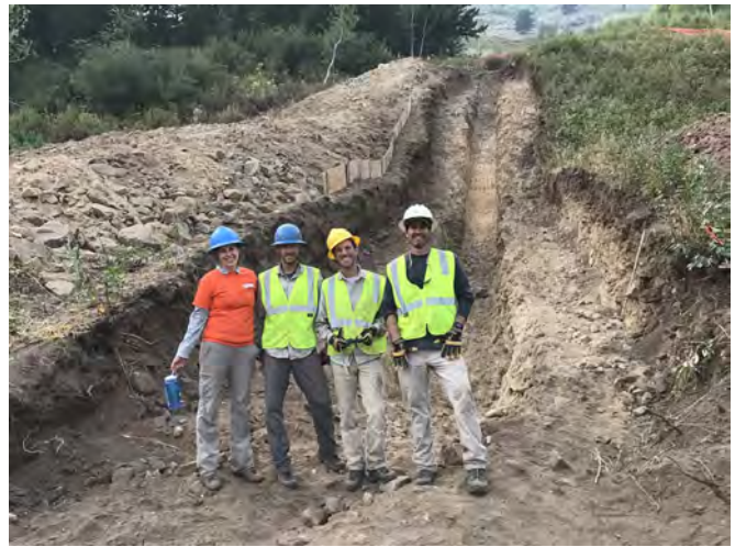
Figure 9.30: Fault trench near Teton Fault. Trenches allow geologists to see a cross section of a fault and to use dating techniques to determine how frequently earthquakes occur.
