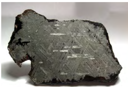
Figure 2.17: A polished fragment of the iron-rich Toluca Meteorite, with octahedral Widmanstätten pattern.
