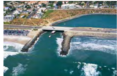
Figure 12.10: Jetties near Carlsbad, California. Notice the left jetty is loaded with sand, while the right jetty is lacking sand. This is due to the longshore drift going left to right.
