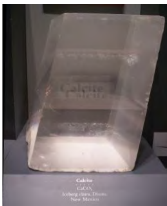
Figure 3.32: Calcite crystal in shape of rhomb. Note the double-refracted word “calcite” in the center of the figure due to birefringence.
