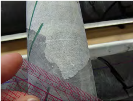
Figure 5.64: A drill core showing a load cast showing light-colored sand sticking down into dark mud.
