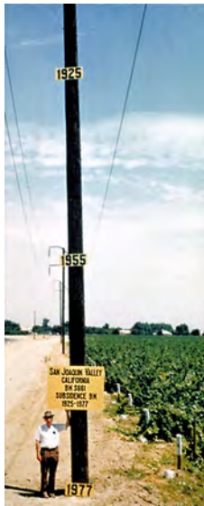
Figure 11.36: Evidence of land subsidence from pumping of groundwater shown by dates on a pole.
