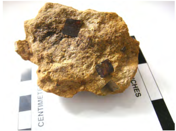
Figure 5.15: Pyrite cubes are oxidized, becoming a new mineral goethite. In this case, goethite is a pseudomorph after pyrite, meaning it has taken the form of another mineral.
