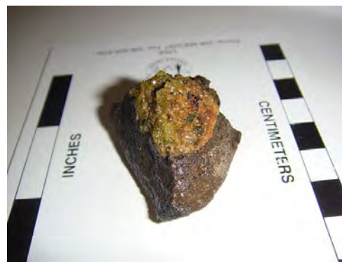
Figure 5.12: This mantle xenolith containing olivine (green) is chemically weathering by hydrolysis and oxidation into the pseudo-mineral iddingsite, which is a complex of water, clay, and iron oxides. The more altered side of the rock has been exposed to the environment longer.
