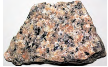
Figure 4.3: Granite is a classic coarse-grained (phaneritic) intrusive igneous rock. The different colors are unique minerals. The black colors are likely two or three different minerals.
