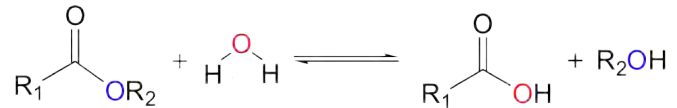
Figure 5.10: Generic hydrolysis diagram, where the bonds in mineral in question would represent the left side of the diagram.
