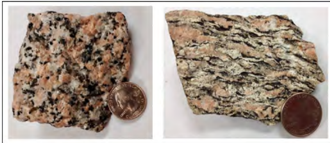
Figure 6.4: An igneous rock granite (left) and foliated high-temperature and high-pressure metamorphic rock gneiss (right) illustrating a metamorphic texture.
