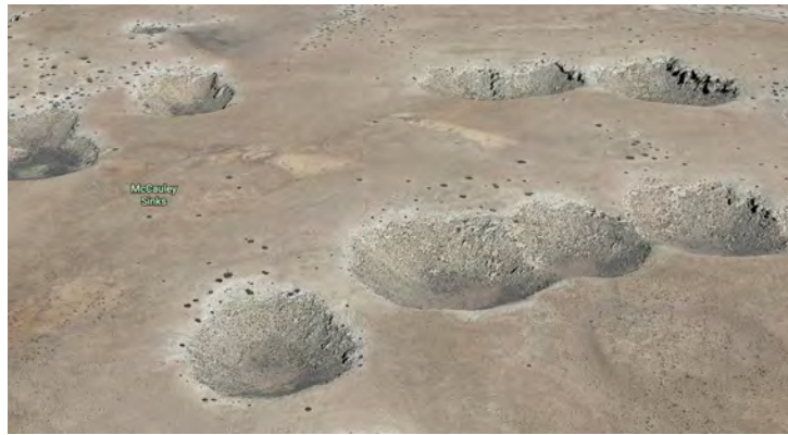
Figure 11.38: Sinkholes of the McCauley Sink in Northern Arizona, produced by collapse of Kaibab Limestone into caverns caused by solution of underlying salt deposits.
