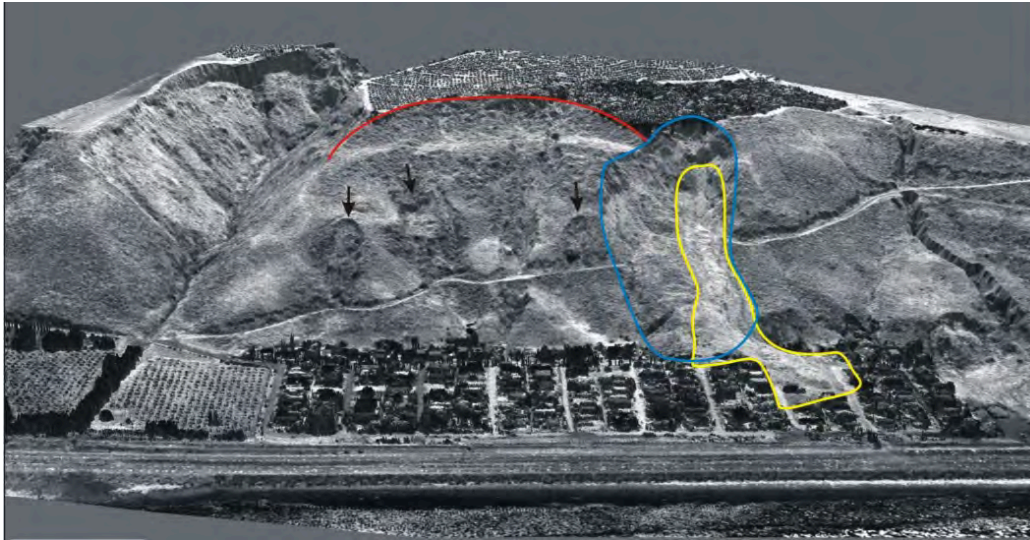
Figure 10.9: Oblique LIDAR image of La Conchita after the 2005 landslide. Outline of 1995 (blue) and 2005 (yellow) landslides shown; arrows show examples of other landslides in the area; red line outlines main scarp of an ancient landslide for the entire bluff.
