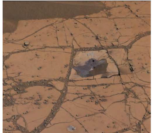
Figure 3.46: The rover Curiosity drilled a hole in this rock from Mars, and confirmed the mineral hematite, as mapped from satellites.
