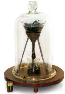
Figure 1.6: An experiment at the University of Queensland has been going since 1927. A petroleum product called pitch, which is highly viscous, drips out of a funnel about once per decade.
