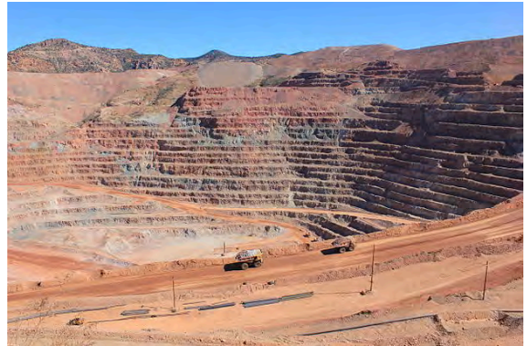
Figure 16.28: The Morenci porphyry is oxidized toward its top (as seen as red rocks in the wall of the mine), creating supergene enrichment.
