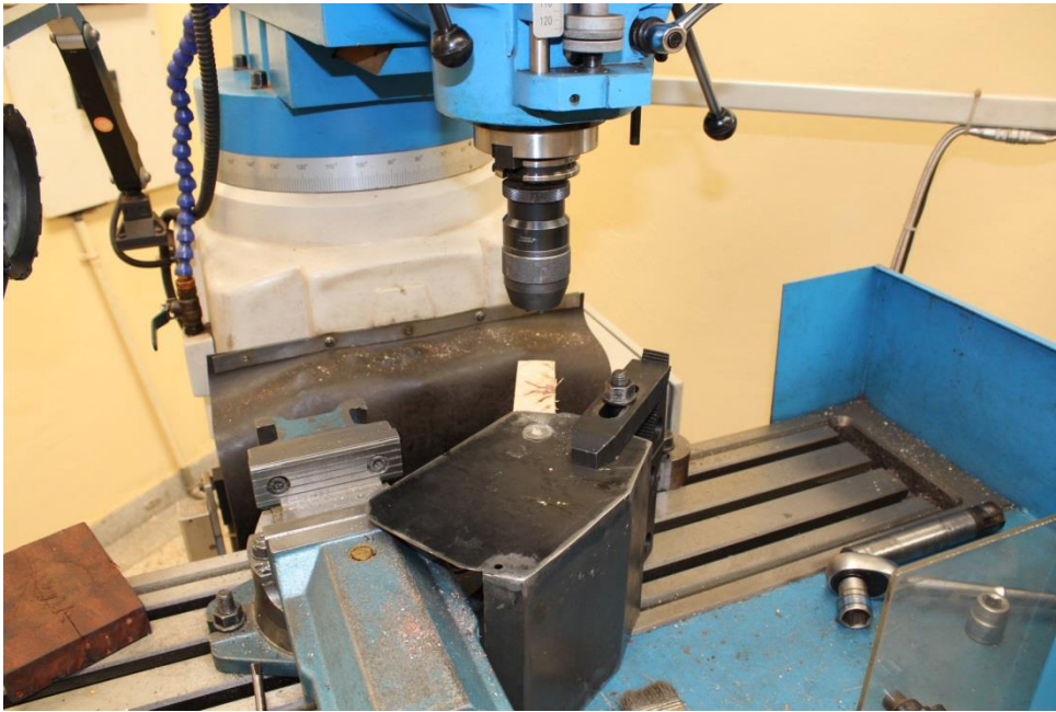
Figure 2: In-house manufacturing of the ECGF user interface
