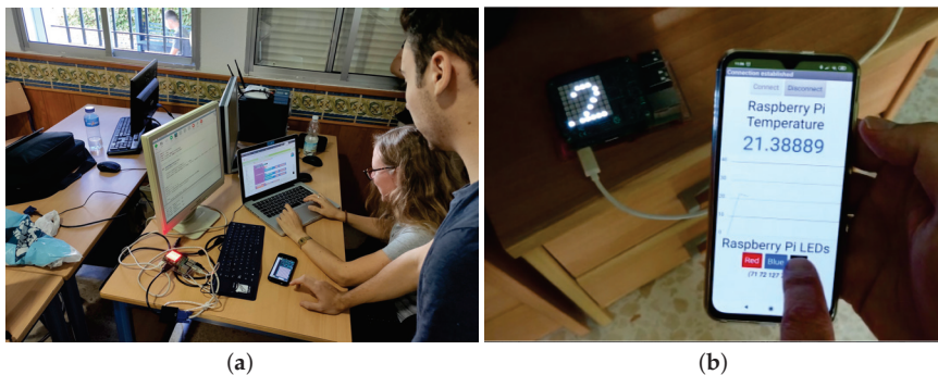
Figure 7. Developing the mobile app for interacting with the external Internet of Things (IoT) device. (a) Students programming the mobile app; (b) Android app communicating with the Raspberry Pi and its Sense HAT add-on.
