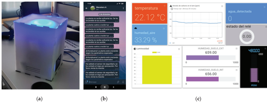
Figure 3. Feedback services configured: (a) Prisma, a visual feedback display; (b) Telegram messenger to receive alerts; (c) IoT cloud platform. Thingsboard.io desktop dashboard.
