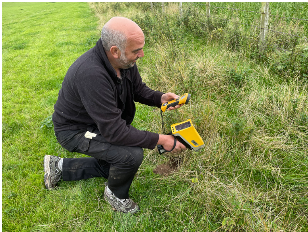
Figure 2. Undertaking simultaneous geochemical and magnetic susceptibility survey in the field using a magnetic susceptibility meter (left hand) and a handheld pXRF machine (right hand).
