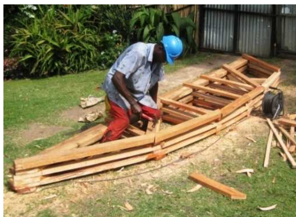
Fig. 28: Once the first mould is constructed, the others are easily copied and shaped with a machete.
