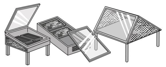
A box dryer is great for home use and for moving around easily from place to place to avoid rain and shade. You can put wheels on the bottom and handles on the outside for even better mobility. If you do not need to move it around you can put legs on it to make it easier to access the food and keep the food further off the ground.
