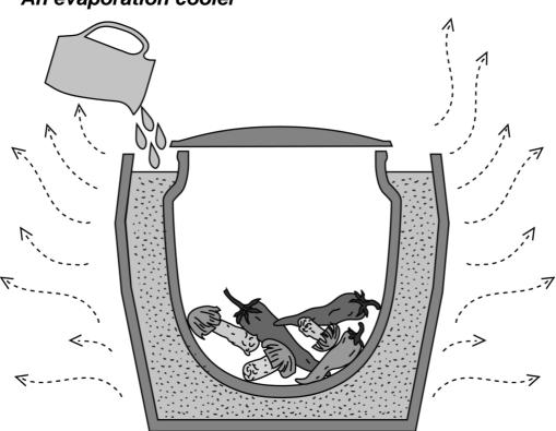
These are perfect for keeping fruits and vegetables fresh for several days. Water is added into clean sand that is between two clay pots and as the water evaporates out, the pots become cool. If you do not have pots, you can use any container or cloth that allows for evaporation. Be creative!
