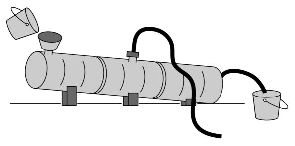
This picture shows a system made from 3 drums. The manure goes in at the top end, the gas rises and is taken away using the pipe in the middle, and the slurry is taken from the other end and used to enrich the soil and strengthen the Nature Cycle. The drums could be on a natural slope instead of a stand. The designs are endless!
