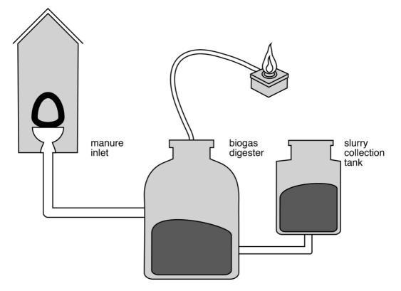
**Organic matter (like manure and fresh plant scraps) is put into a 'digester'.** Water is added. The digester works like a stomach to digest food. There are many different ways to put this material in the digester. It can be a part of the regular sewage system or there can be a door or opening to add the organic matter (then close it again so the gas does not escape). Organic matter should be added often so that gases are always being made. Water will need to be added too.
