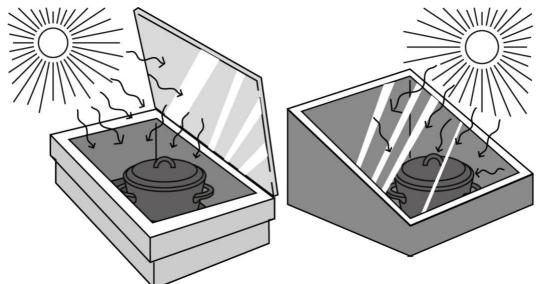
The top of the box is covered with glass or clear material that can allow sunlight to enter the box and trap heat. The inside of the box should be black, ideally, to absorb heat. An adjustable reflector can be attached to the top of the box to direct more heat and light onto the pot
