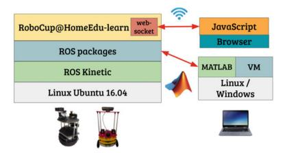
Fig. 2 Example of development architecture
