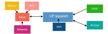
Fig. 2 Simplified diagram of the electronics of Erwhi Hedgehog
