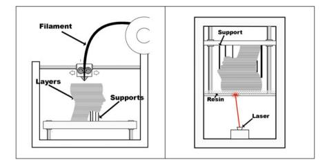
Fig. 1 FDM (right) and SLA (left) 3D printing technologies
