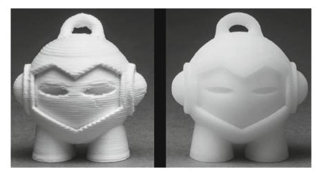
Fig. 2 The same object printed with FDM (left) and SLA (right). *Source* https://www.3dhubs.com/ knowledge-base/key-design-considerations-3d-printing
