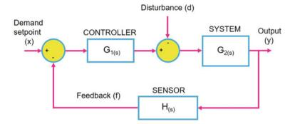
Fig. 2 General diagram of the feedback control system
