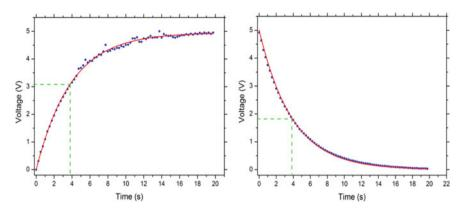
Fig. 2 Charge (left) and discharge (right) process of an *RC* circuit:  $R = 3850 \ \Omega$  and  $C = 1 \ \text{mF}$ . The theoretical time constant is  $\tau = RC = 3.85 \ \text{s}$ . The experimental values are, respectively,  $\tau = (3.87 \pm 0.08) \ \text{s}$  and  $\tau = (3.83 \pm 0.08) \ \text{s}$ . Experimental data (blue dots) are fitted with an exponential curve (red solid line)
