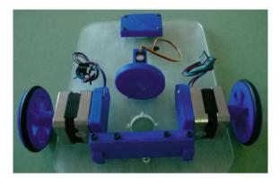
Fig. 1 First vehicle chassis
