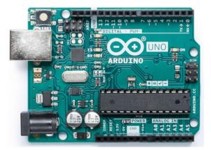
Fig. 1 Front view of Arduino Uno board. Analog pins are numbered from A0 to A5 (bottom right), whereas digital pins go from 0 to 13 (top row). The symbol "  $\sim$  " denotes pins that can deliver an analog voltage by means of the pulse width modulation (PWM) technique
