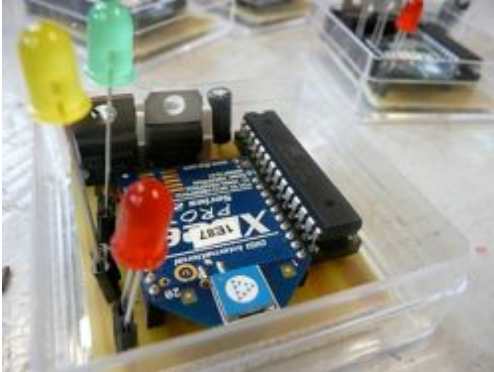
23 HC Gilje, Arduino-Standalone with Xbee for Wind-Up Birds , 2007, Xbee, ATmega 168 microchip, solenoid with wooden box and metal roof, (photograph provided by: HC Gilje)
