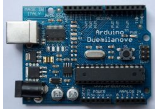
3 Arduino microcontroller , 2008, 2.7 in. x 2.1 in. (Photograph provided Nicholas Zambetti)
