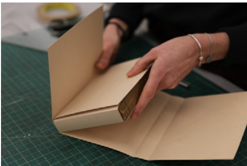
Placing the wrapped book onto the horizontal strip.
