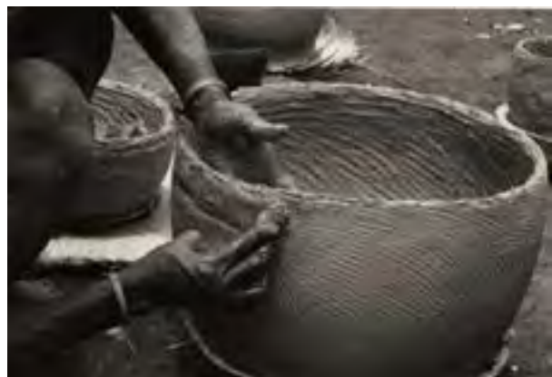
FIG. 24. This Gbaya potter from Cameroon has added a coil of clay to the top of the pot, and is flattening and smoothing it into the existing clay. © The Trustees of the British Museum, Af,CB63.10. Creative Commons CC BY-NC-SA 4.0.
